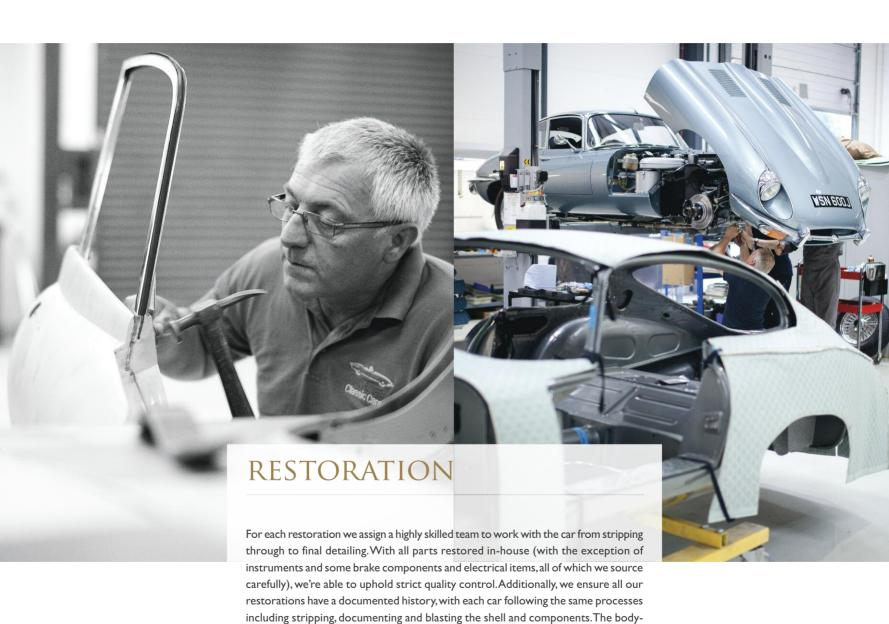
work is restored in-house on custom built jigs before being moved to the paint preparation area, where the car is fully pre-fitted to ensure all panel gaps are correct and components fit perfectly. With strict approved supplier criteria, we send our
